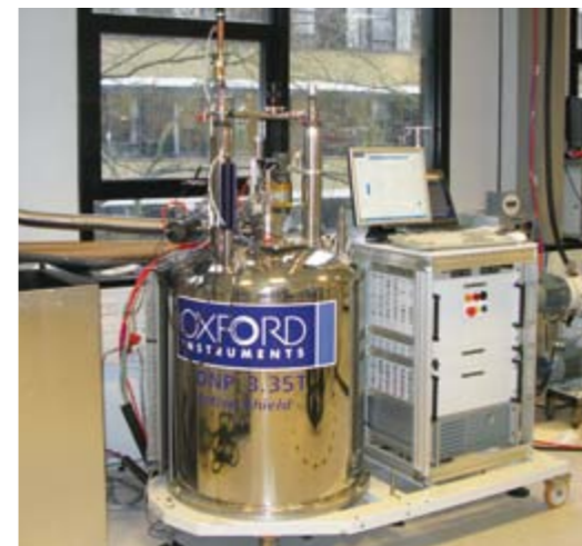
Magnet at work: The DNP magnet at DTU Electrical Engineering polarise the electron spin of the radical.
