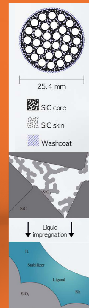
Schematic drawing and photograph of the cylindrical porous monolith consisting of a SiC core, SiC skin, and silica wash-coat. Detailed schematic drawing of the pore structure before and after liquid impregnation.
