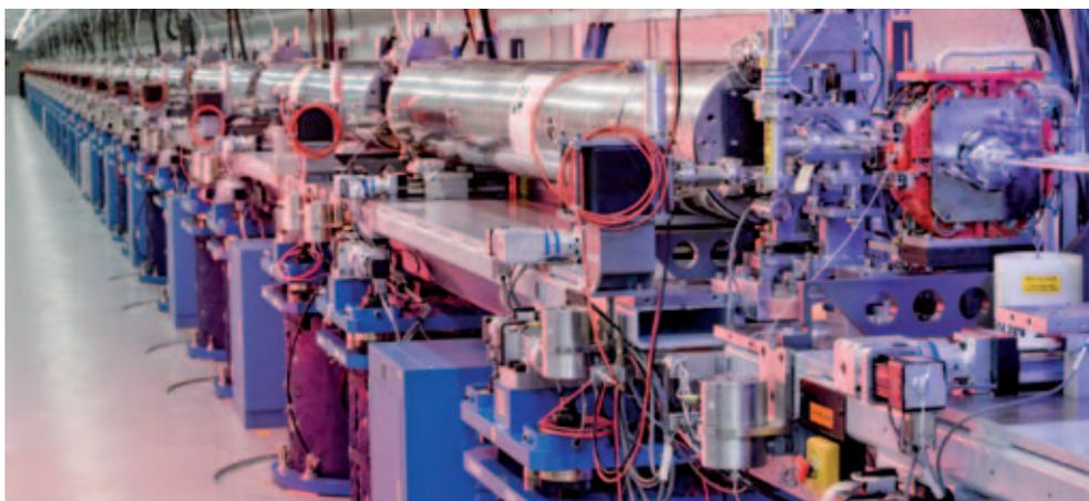
*Looking east down the LCLS undulator array. Thirty-three LCLS undulator magnets will create intense X-ray laser light from a pulse of electrons traveling near the speed of light.*
