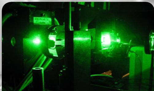
**Raman Spectroscopy** is an universal analytical technique for identification of molecules in gases, liquids and solids by scattering of laser light. The Department has recently obtained a new confocal Raman instrument associated with a microscope and fiber optics.
