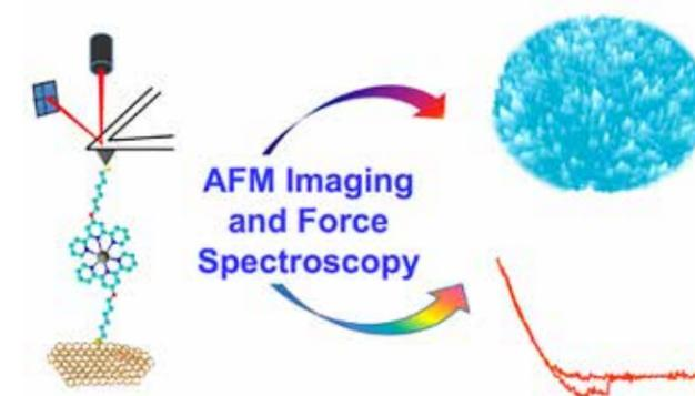
When the atomic force microscope (AFM) tip approaches the sample, tip-bound terpy interacts with Os-terpy on the substrate surface to form the complex. Retraction of the tip results in dissociation of the Os-terpy bond but does not break the Au-S bond, which is much stronger than the coordinative bond. Force-distance curves for the Os-terpy ligand dissociation process can thus be recorded.
