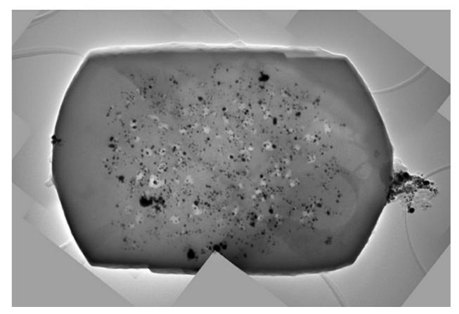
TEM image of gold nano particles encapsulated in a zeolite crystal. The black areas represent high density regions, and therefore correspond to the gold particles. The image and the sample were made by researchers from Haldor Topsøe in collaboration with DTU (published in Angew. Chem. Int. Ed. 2010, 49, 3504 - 3507)
