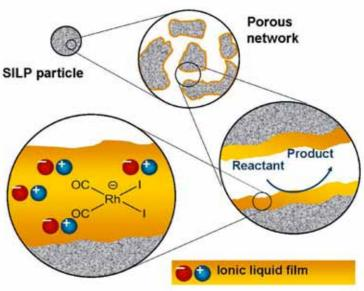
The main attraction of the SILP process is that it allows for a steady production of acetic acid without having to stop and restart the reaction. Continuous flow production is attractive for a number of reasons. One of them is smoother quality assurance compared with traditional batch production, which often involves complex procedures between batches. Also, in some cases continuous production can be cheaper.
