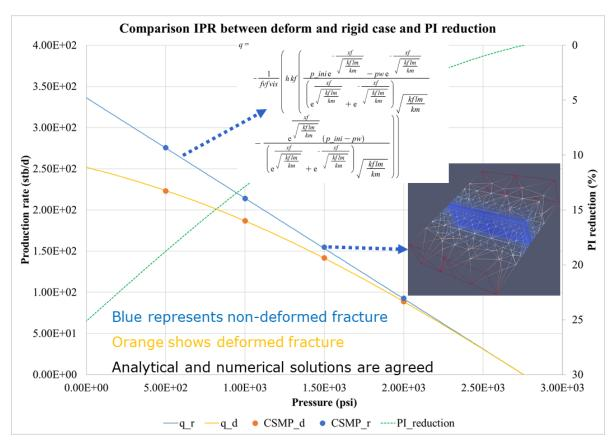
Figure 1 Steady-state production comparison between analytical and numerical solutions
