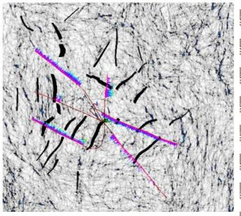
Ant-tracked seismic volume at top reservoir, well-scale fracture densities (purple) and structural framework (black).
