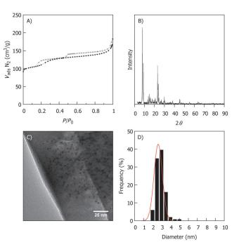
**Figure 2.** A)  $N_2$  physisorption isotherm of Au/Recryst-S1 at 77 K. B) XRD pattern of Au/Recryst-S1 (MFI crystal structure). C) TEM image of Au/Recryst-S1. D) Size distribution based on measurements of approximately 250 nanoparticles by TEM.
