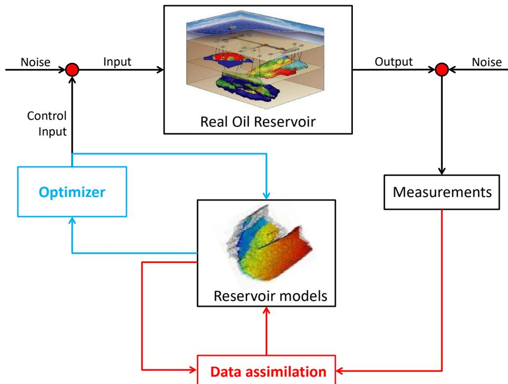
Fig. 1: Diagram illustrating the role of optimal control (the blue loop) in a production optimization workflow (known as closed-loop reservoir management).
