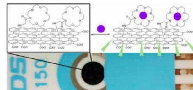
Crown-ether functionalized graphene nanosheets and sensor for selective sensing of potassium ions.
